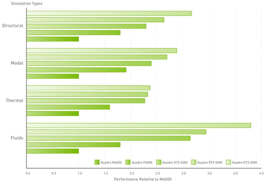
Tests run on a workstation with Intel Xeon Gold 6154 3.0GHz (3.7GHz Turbo), 18 cores, 36 threads, 24.75MB cache, 64GB RAM DDR4, Windows 10 RS4, NVIDIA Driver 417.04. Performance testing completed with a range of models for each simulation type using ANSYS Discovery Live. \*Fluids only available in ADL.
