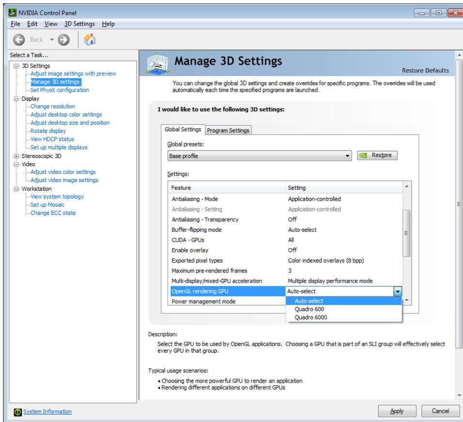
Figure 13. Setting Render GPU from NVIDIA Control Panel
