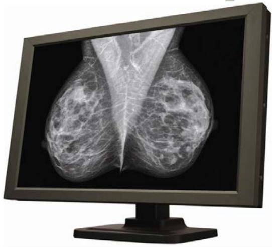
Figure 1. 10 MPixel 10-Bit Diagnostic Mammography Display<sup>1</sup>
