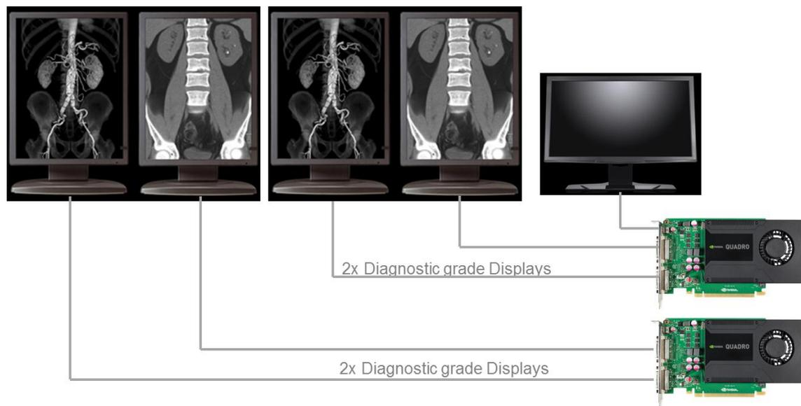
Figure 4. Three GPUs Driving a 20 MP Grayscale Display
