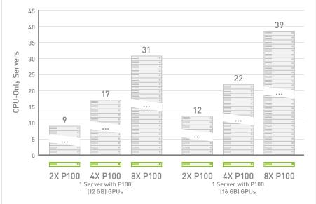
CPU Server: Dual Xeon E5-2690 v4 @ 2.6GHz, GPU Servers: Same as CPU server with NVIDIA\* Tesla\* P100 for PCIe (12 GB or 16 GB) | NVIDIA CUDA\* Version: 8.0.44 | Dataset: 256x256 x256 local size | To arrive at CPU node equivalence, we use measured benchmark with up to 8 CPU nodes. Then we use linear scaling to scale beyond 8 nodes.
