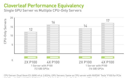
(12 GB or 16 GB) | NUDIA CUDA" Version: 8.0.44 | Dataset: bm32 | To arrive at CPU node equivalence, we use measured benchmark with up to 8 CPU nodes. Then we use linear scaling to scale beyond 8 nodes.
