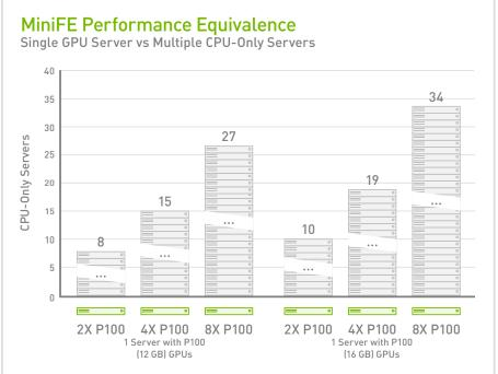
CPU Server: Single Xeon E5-2690 v4 @ 2.6GHz, GPU Servers: Same as CPU server with NVIDIA" Tesla" P100 for PCle (12 GB or 16 GB) | NVIDIA CUDA" Version: 8.0.44 | Dataset: 350x350x350 | To arrive at CPU node equivalence, we use measured benchmark with up to 8 CPU nodes. Then we use linear scaling to scale beyond 8 nodes.
