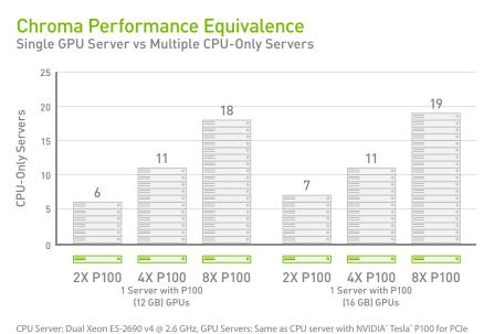
CPU Server: Dual Xeon E5-2690 v4 @ 2.6 GHz, GPU Servers: Same as CPU server with NVIDIA" Tesla" P100 for PCIe (12 GB or 16 GB) | NVIDIA CUDA" Version: 8.0.44 | Dataset: szscl21\_24\_128 (total time sec) | To arrive at CPU node equivalence, we used measured benchmarks with up to 8 CPU nodes and linear scaling beyond 8 nodes.
