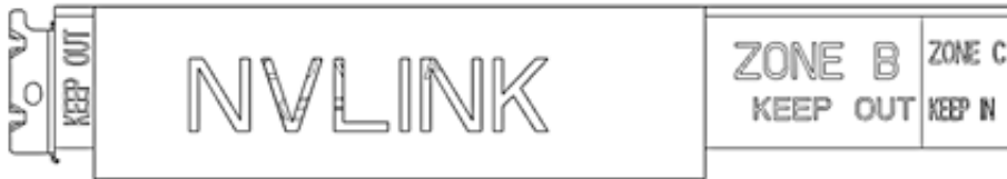
Figure 5. NVLink Connector Placement – Top View
