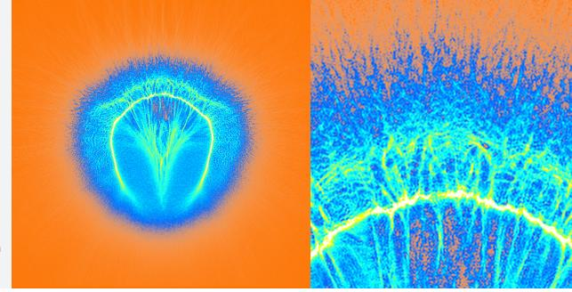
**Right:** Ions in a micron-sized spherical target after a high power laser has hit. Source: TU Dresden.
